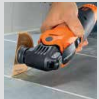
At just 1.2 mm wide, the saw blades can cut out even very narrow joints.
