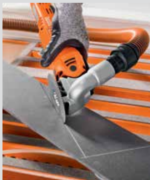
Cuts in carbon fibre materials.
