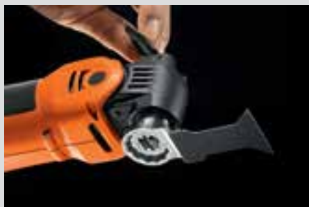
To release, open clamping lever ...
