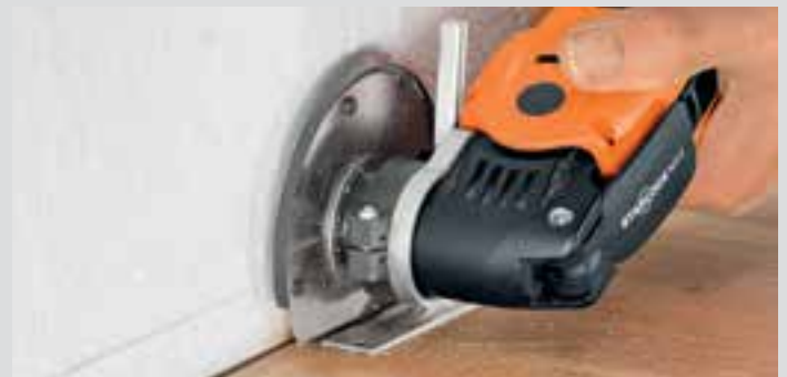
Perfect recutting of expansion joints.
