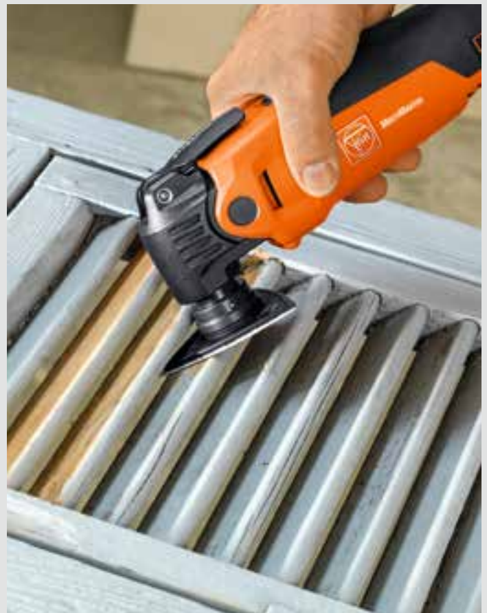
Tynn slipeplate for smale mellomrom.
