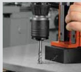
Tapping with fast change tapping chuck
