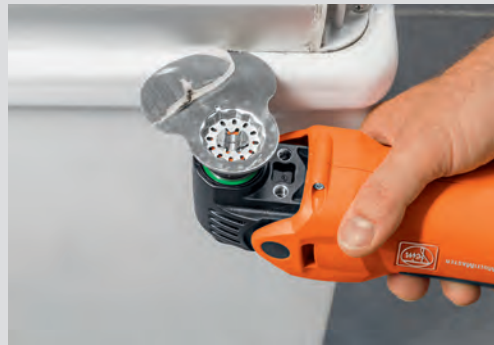
Remove connection joints.
