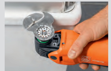
Remove connection joints.
