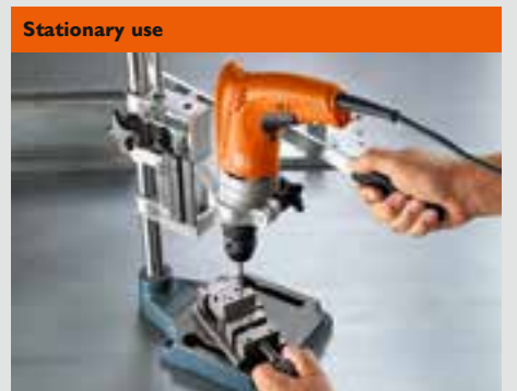
The standardised Euro collar means that all the drills can also be used for stationary work.
