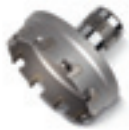
Carbide hole saw with QuickIN PLUS holder Carbide cutting tips for optimum service life for efficient drilling in sheet metal plate up to 4.0 mm thick. Imperial dimensions, cutting depth 4 mm/ 5/32".
