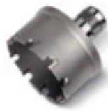
Carbide hole saw for pipes with QuickIN PLUS holder Carbide cutting tips for optimum service life for use with pipe material and curved surfaces with wall thicknesses of up to 4 mm. Metric dimensions, cutting depth 4 mm.
