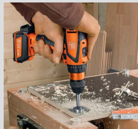
Ideal for assembly work, e.g. installation of European hinges with a Forstner bit.
