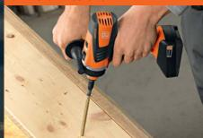
Even demanding screw connections such as  $3\% \times 15^{-3}\%$  in (10 x 400 mm) fully threaded screws go smoothly without pre-drilling.
