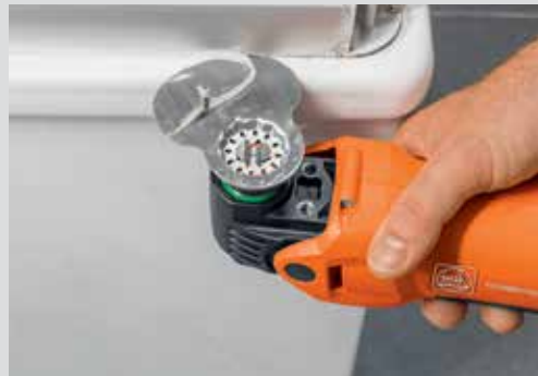
Remove connection joints.
