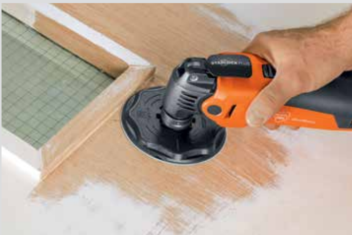
The large sanding disc replaces additional sanding machines such as random orbit or pad sanders.
