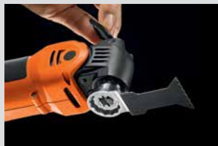
To release, lift the locking lever.
