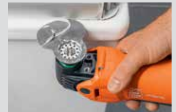
Remove connection joints.
