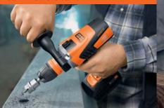
Drilling large hole diameters in 1st or 2nd gear. Torque setting 15 provides additional safety when stalling.
