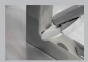
Fillet welds can be polished to a mirror polish using the felt disc and polishing paste.
