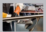
Tarnishing can be quickly removed without damaging neighbouring components by using the (fine) fleece disc.
