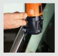
Use the 25.4 and 19 mm 207 and 208 L-blades for narrow gaps (min. 3 mm). The short design means you don't have to dismantle the interior coverings on the A-columns.
