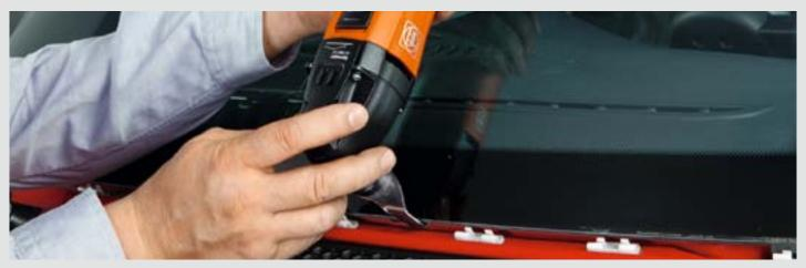
Use the U-blades to remove glass from under the bonnet. Recommended speed: level 3-5.
