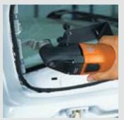
In some VAG models, the rear and side windows are fitted with moulded frames. FEIN provides you with the perfect solution for removing the windows in the VW Passat variant models up to 2004, from the VW Polo to the 01, Lupo, Seat and VW Golf III, without causing any damage.
