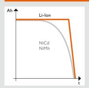
Powerful from the first cut to the last: the new FEIN lithiumion technology delivers constant power until the battery is completely flat.
