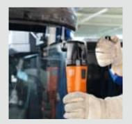
When it comes to hard-to-reach bonds, e.g. under sun visors or for permanently fitted display panels in buses, the reinforced blade, form 217, is ideal. Recommended speed: level 4-5.
