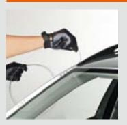
The wire is simply rolled under the moulded strips – preventing these from being damaged during removal and allowing the window to be reused.
