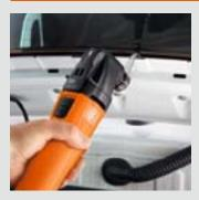
Glass can be removed from encapsulated side windows and rear windscreens from the inside using the L-blades, available in three different lengths up to 38 mm.
