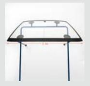
5–6 times the total width of the window at the bottom is sufficient for the wire length. Wire which is 2–2.5 times the inner width of the vehicle therefore needs pulling into the interior with the awl.
