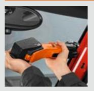
If the outer gap between the glass and bodywork is less than 3 mm, the window must be cut out from the inside using a straight blade. **Recommended speed:** max. level 3.
