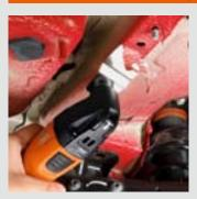
The stopper knife allows you to remove underseal and stoneguard with ease and at speed. Parts needing repair can be easily exposed and e.g. tow couplings screwed directly to the framework.
