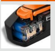
Thanks to the sophisticated electronics, all cells are individually monitored and therefore reliably protected from overload, overheating and total discharge.
