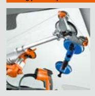
In rare cases the telescopic arm may slip on the window. This can be avoided by using a standard lifting pad.
