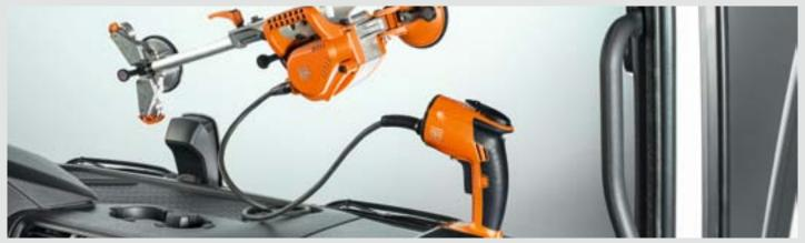
Glass can be reliably removed from truck windscreens by repositioning the SUPERWIRE just once. Start by positioning the SUPERWIRE on the right-hand side of the vehicle, cutting normally until the machine wire reaches the centre on the windscreen. The windscreen can be cut out to roughly the centre of the headliner. Then the SUPERWIRE has to be moved over to the left.
