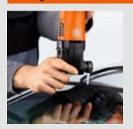
Encapsulated windscreens and moulded frames, also with aluminium reinforcement, can be cut out with the L-blade in a single step. **Recommended speed: level 3–4.**
