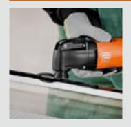
The mushroom-shaped cutter blade cuts out insulation windows from buses and trains with ease and at speed. Adhesive residue on the glass can therefore also be removed with ease.
