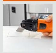
The wide or narrow M-CuT HSS saw blades allow you to make cut-outs in fibreglass and other plastic composites with precision.
