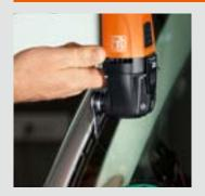
The L-blade provides a 40% higher cutting performance compared with a U-blade when used at the same speed. Damage to the bodywork is virtually eliminated. **Recommended speed: level 3–4.**
