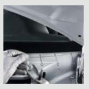
If the window extends over the body flange, we would recommend using metal stakes to ensure that the wire is in contact with the window when cutting.
