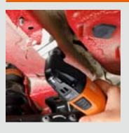
The stopper knife allows you to remove underseal and stoneguard with ease and at speed. Parts needing repaired can be easily exposed, and tow couplings screwed directly to the framework. Interior carpets, sound-deadening mats and insulation mats can also be removed with ease.
