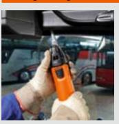
Even very large windows can be cut out with ease from the inside with the cutter blade, form 081. **Recommended** speed: level 3–5.
