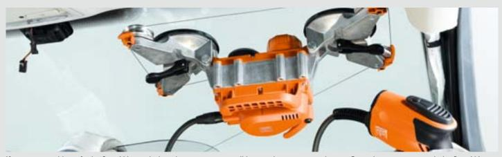
If you are not able to fit the SUPERWIRE with the telescopic arms, it will have to be repositioned once. Once the wire is inserted, the SUPERWIRE is secured in the top right. The windscreen is cut out up to the top edge, then the SUPERWIRE is moved to the left to remove the rest of it.
