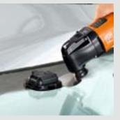
The new range of accessories is also suited to other tasks. The mushroom blade can be used to remove with ease e.g. the light and windscreen wiper sensors, which are a common feature in modern vehicles.
