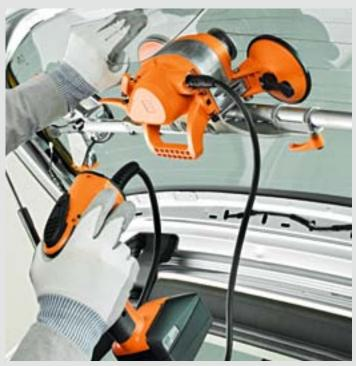
On low rear windscreens, e.g. in estate cars, the  $\mbox{\sc SuperWire}$  is fitted in parallel on the windscreen.
