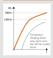
Shortened charge time: high-quality battery cells with low internal resistance reduce heat build-up and the battery doesn't have to be cooled at outdoor temperatures of up to 45 °C.
