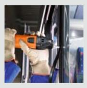
Joints in bus windows have to be removed with a V-cut before the window can be cut out. Its fast cut makes the straight cutter blade, form 073, optimally suited to the task.
