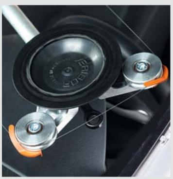
If the windscreen is so curved that a lifting pad cannot stick to the windscreen, this can be compensated for by fitting the vacuum ring.
