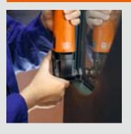
The curved cutter blade, form 072, is excellently suited to making separating cuts in side windows from inside.
