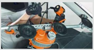
Thanks to motorisation, the SuperWire can be effortlessly controlled from inside or outside by remote control.
