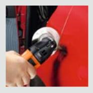
The HSS saw blades allow you to cut rapidly through normal-strength bodywork sheet metal up to 1 mm, hard plastics and fibreglass. The cutting line is only 0.5 mm wide. You also benefit from spark-free cutting and individual immersion depths into the material.
