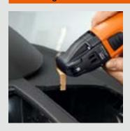
The carbide-tipped file is optimally suited to reworking cut-outs in hard-to-reach places: it makes light work of plastics, composite material and wood.
