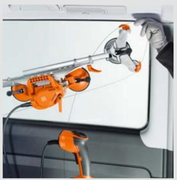
Glass can also be easily removed from larger side windows without the need to reposition. Always start to insert the wire in the top right.
