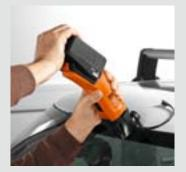
Encapsulated windscreens and moulded frames, also with aluminium reinforcement, can be cut out with the L-blade in a single step. **Recommended speed: level 3–4.**
