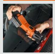
The reinforced U-blade is used to remove glass from under the bonnet. **Recommended** speed: level 3-4.
