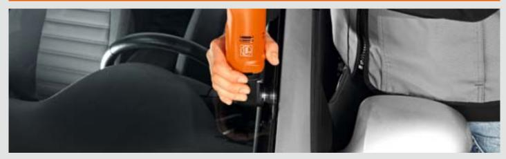
It makes an extremely fast cut! The L-blade, form 207, has a 40% higher cutting performance compared with a U-blade when used at the same speed setting. This is a major benefit when removing glass from windscreens from outside the vehicle. **Recommended speed: level 3-4.**
