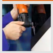
Bonded cover strips can be removed cleanly, reliably and at speed with the straight blades, form 081 and 216, enabling the strips to be reused in most cases. **Recommended speed:** level 3–5.
