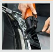
The scraper blade allows you to remove residual adhesive cleanly, at speed and with little effort. Recommended speed: level 2-3.
