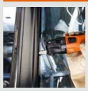
Stage-bonded or U-profile bonded windows can even be cut out at the edges with the cutter blade, form 177, with an angle cutter of 8 mm. Best suited to bus and train windows.
