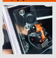
The LED lighting in the remote control and the transparent covers allow the path of the cutting wire to be followed at all times.
