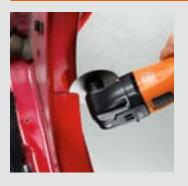
The HSS saw blade allows you to cut bodywork sheet metal up to 1 mm rapidly and without producing sparks, as well as most plastics and fibreglass. The cutting width is only 0.5 mm. Not suited to high-strength bodywork sheet metal. Recommended speed: level 3–5.
