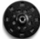
Sanding pad With hook and loop fastening, Ø 150 mm with M 14 suction hole. Hole circle suitable for FEIN and other sanding materials.
