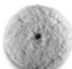
Lamb's wool, dome shape Diameter approx. 230 mm for backing pads with a Ø of 170 mm, 6 38 06 187 01 0, M 14 with hook and loop fastening system. Recommended working speed 500-1 200 rpm. Quality TOPWOOL, fleece polishing wheel. Lamb's wool/synthetic blend, washable.
