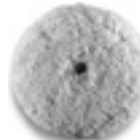
Lamb's wool, dome shape Diameter approx. 230 mm for backing pads with a Ø of 170 mm, 6 38 06 187 01 0, M 14 with hook and loop fastening system. Recommended working speed 500-1 200 rpm. Quality TOPWOOL, fleece polishing wheel. Lamb's wool/synthetic blend, washable.
