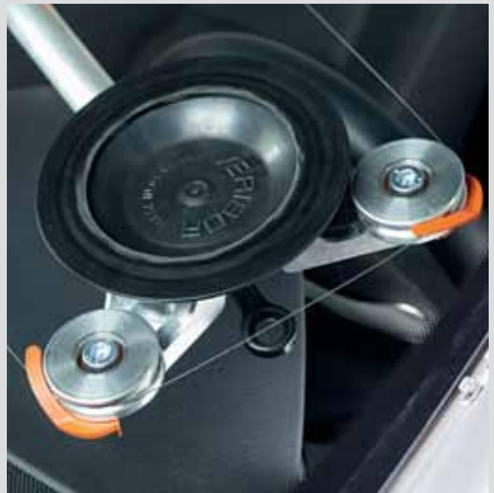
If a suction cup does not stick to the window because of window curvature, installing the vacuum ring can compensate.
