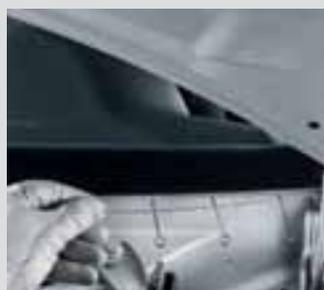
If the window extends over the body flange, use of metal pins is recommended so the wire is against the glass when cutting.
