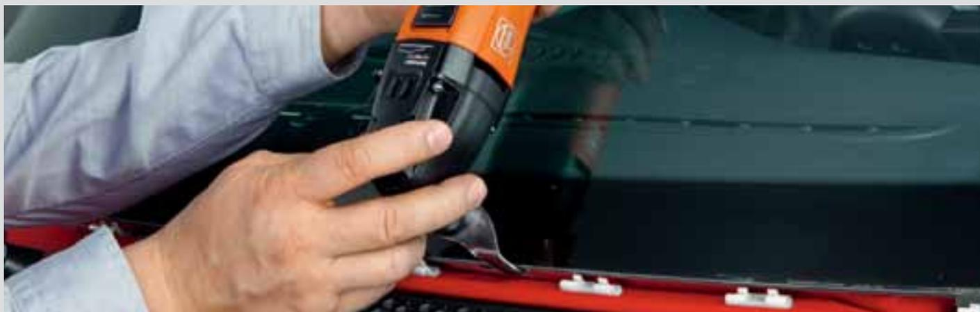
The U-shaped blades are used for glass removal below hood level. Recommended speed: setting 3–5.
