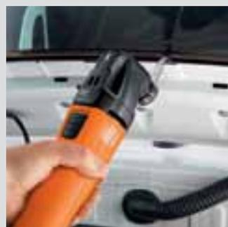
Encapsulated side and rear windows can be removed from the inside using L-shaped blades in three different lengths up to 1 1/2" (38 mm).
