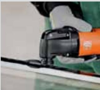
The mushroom-shaped cutter blade separates bus and rail vehicle insulating glass panes effortlessly and quickly. It can also be used to easily remove adhesive residue from glass.
