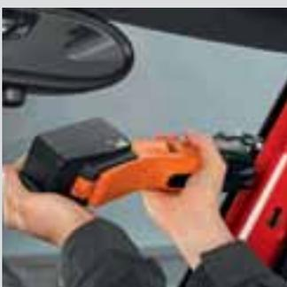
If the gap between glass and auto body is less than 1/2" (3 mm), the windshield must be cut out from the interior using a straight blade. Recommended speed: max. setting 3.
