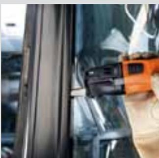
Windows glued into rabbets or U-shaped moldings can be cut out with the type 177 cutter blade which has an angled  $\frac{5}{16}$ " (8 mm) cutting edge and can even cut along edges. Excellent for bus and rail vehicle windows.
