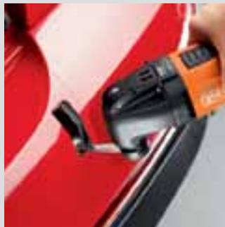
The type 081 toothed straight cutter blade is ideal for removal of glued plastic and add-on parts such as trim or body molding. The type 073 cutter blade is perfect for subsequent cutouts such as those in plastic bumpers.
