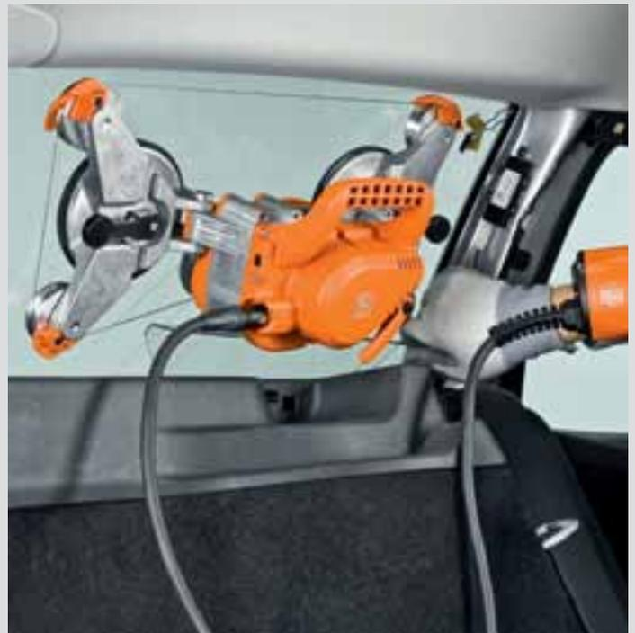
By removing the telescoping unit and installing the guide rollers directly on the drive unit, small side windows can also be removed without repositioning.
