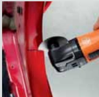
With the HSS saw blade, you can cut auto body sheet metal up to 1/32" (1 mm) speedily and spark free as well as most plastics and GRP. The kerf is a mere 1/64" (0.5 mm). Not suitable for high-tensile body sheet metal. Recommended speed: setting 3–5.
