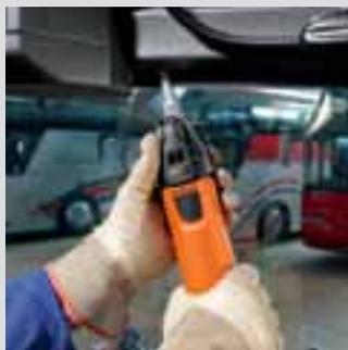
Even very large windows can be cut out from the interior using a type 081 cutter blade. Recommended speed: setting 3–5.
