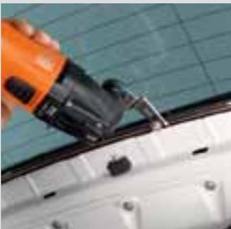
Side and rear windows are easily and quickly removed from the interior using the type 143 cutter blade and the adjustable depth stop. Recommended speed: max. setting 3.
