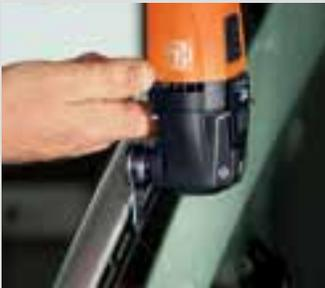
The 1" (25.4 mm) type 207 and 3/4" (19 mm) type 208 length-shaped blades are used on narrow gaps (min. 3/32"/3mm). The short shape can avoid the need to remove interior pillar trim.
