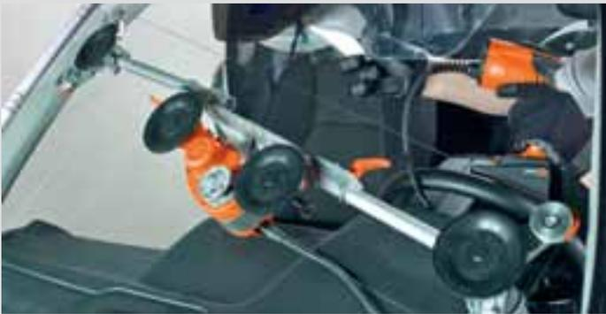
The SUPERWIRE is easily mounted and operated. The unit is not repositioned during the entire process of glass removal. This ensures that the work does not need to be interrupted.
