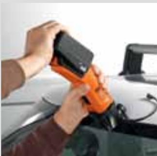
Encapsulated windshields and molded frames, including those with aluminum reinforcement, can be removed in one step using the L-shaped blade. Recommended speed: setting 3–4.
