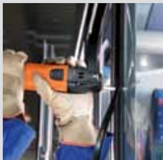
Joint fillers on bus windows must be removed with a V cut before the window can be removed. The straight type 073 cutter blade is ideal for this due to its very rapid cutting ability. Recommended speed: setting 3–5.
