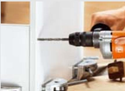
Drilling holes in composite material is no problem, due to high rpm.
