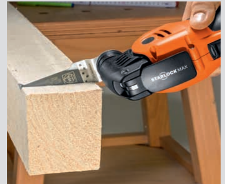
Even heavy construction lumber can be effortlessly cut to length with the SUPERCUT.
