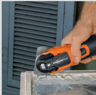
Oscillation motion eliminates risk of glass breakage.
