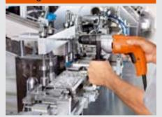
Fast work progress and optimal concentricity for precision work using the inline grip.
