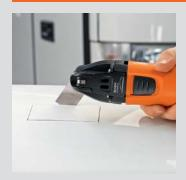
Cutouts in GRP and other resin-based materials can be precisely executed with the wide or narrow M-Cut HSS saw blades.
