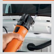
Encapsulated side and rear windows can be removed from the inside using L-shaped blades in three different lengths up to 1 ½" (38 mm).
