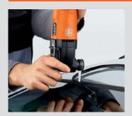
Encapsulated windshields and molded frames, including those with aluminum reinforcement, can be removed in one step using the L-shaped blade.
