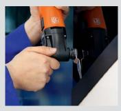
The type 081 and 216 straight blades remove cover strips neatly, safely, and quickly. In most cases, this allows the strips to be reused. Recommended speed: setting 3–5.
