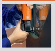
The curved type 072 cutter blade is ideally suited to cutting out side windows from the interior. Recommended speed: setting 3–4.
