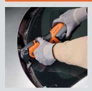
The heavier U-shaped blade is used for glass removal below hood level. Recommended speed: setting 3-4.
