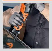
Encapsulated windshields and molded frames, including those with aluminum reinforcement, can be removed in one step using the L-shaped blade.
