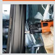
Windows glued into rabbets or U-shaped moldings can be cut out with the type 177 cutter blade which has an angled 5/16" (8 mm) cutting edge and can even cut along edges. Excellent for bus and rail vehicle windows.
