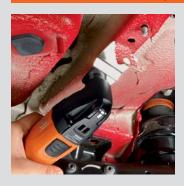
Remove underseal and stone damage protection easily and quickly with the rigid scraper blade. This allows repair locations to be exposed easily and tow hitches to be bolted directly to the frame. Recommended speed: setting 2–4.
