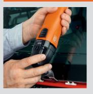
The U-shaped blades are used for glass removal below hood level. Recommended speed: setting 3–5.
