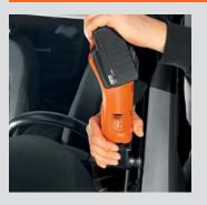
Extremely fast cutting: the type 207 L-shaped blade has an approximately 40% better cutting performance than a comparable U-shaped blade at the same speed setting. This is a great benefit when removing windshields from the outside. Recommended speed: setting 3–4.
