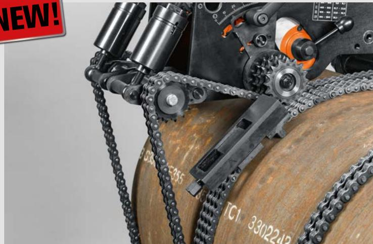
**Precise cutting guidance:** The three chains guarantee that cuts are absolutely straight with no misalignment.
