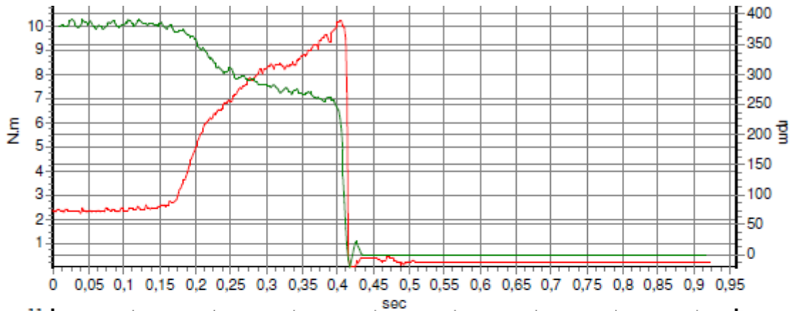
Illustration 19: 360° soft joint 10,2 Nm before load change machine 2017-05.014394
