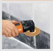
diamond or carbide saw blades with an extra large diameter are available for maximum tool life and cutting speed. Because they are twisted, they achieve a considerably longer service life than segmented blades.
