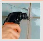
Excellently suited to cutting out particularly hard tile joints such as extremely waterproof epoxy resin joints in swimming pools.
