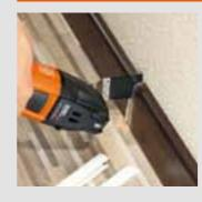
behind the workpiece. Subsequent cut-outs, for example in fitted skirting boards, can be made at speed and with precision.
