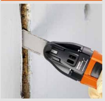
The diamond cleaning blade cleans and roughens mortar flanks before you fill them in again, guaranteeing optimum adhesion of the new sealant material.
