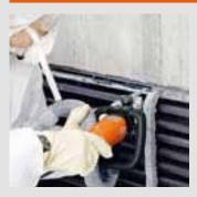
The FEIN SUPERCUT allows you to remove the sealant material, producing minimal dust, with a fitted extraction device.
