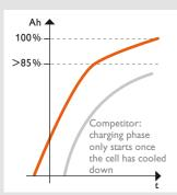
Shortened charge time: heat build-up is reduced thanks to high-quality battery cells with low internal resistance and the battery doesn't have to be cooled at outdoor temperatures of up to 45°C.
