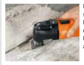
New floorings need a clean surface. The enlarged stopper knife allows you to quickly remove even stubborn residue left behind by old floor coverings and adhesive.
