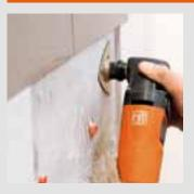
The carbide rasp can remove tile adhesive, plaster and screed, enabling the replacement tile to be quickly fitted.
