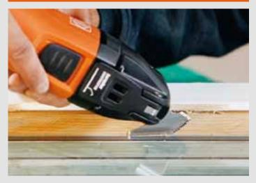
Putty-mounted insulation windows can be removed on-site in one piece without the windows having to be broken up using the segment-shaped cutter blade. This means there's practically no risk of injury, no time-consuming tidying up and you cut working time by up to 80%.
