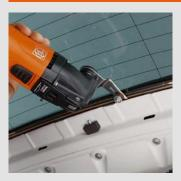
Remove glass from the side and rear windows with ease and at speed with the cutter blade, form 143, and the adjustable stop roller. **Recommended speed: max. level 3.**
