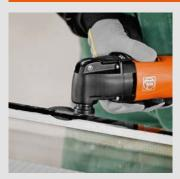
The mushroom-shaped cutter blade cuts out insulation windows from buses and trains with ease and at speed. Adhesive residue on the glass can therefore also be removed with ease.
