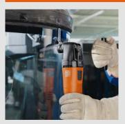
When it comes to hard-toreach bonds, e.g. under sun visors or for permanently fitted display panels in buses, the reinforced blade, form 217, is ideal. Recommended speed: level 4-5.
