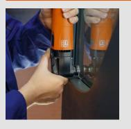
The curved cutter blade, form 072, is excellently suited to making separating cuts in side windows from inside. **Recommended speed:** level 3-4.
