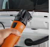
Glass can be removed from encapsulated side windows and rear windscreens from the inside using the L-blades, available in three different lengths up to 38 mm.
