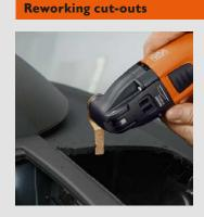
The carbide-tipped file is optimally suited to reworking cut-outs in hard-to-reach places: it makes light work of plastics, composite material and wood.
