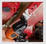
The stopper knife allows you to remove underseal and stoneguard with ease and at speed. Parts needing repair can be easily exposed and e.g. tow couplings screwed directly to the framework. **Recommended speed: level 2–4.**
