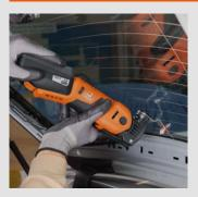
The blade, with form 143, features an adjustable stop roller. This allows windows to be removed quickly and easily from the inside. **Recommended speed: max.** level 3.
