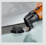
The new range of accessories is also suited to other tasks. The mushroom blade can be used to remove with ease e.g. the light and windscreen wiper sensors, which are a common feature in modern vehicles. **Recommended speed: level 2–3.**
