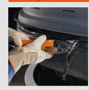
The scraper blade allows you to remove residual adhesive cleanly, with ease and at speed even in hard-to-reach places.
