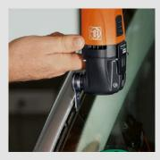
The L-blade provides a 40% higher cutting performance compared with a U-blade when used at the same speed. Damage to the bodywork is virtually eliminated. **Recommended speed: level 3–4.**
