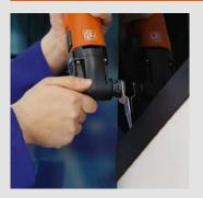
Bonded cover strips can be removed cleanly, reliably and at speed with the straight blades, form 081 and 216, enabling the strips to be reused in most cases. Recommended speed: level 3-5.
