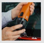
Use the U-blades to remove glass from under the bonnet. **Recommended speed:** level 3–5.
