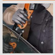
Encapsulated windscreens and moulded frames, also with aluminium reinforcement, can be cut out with the L-blade in a single step. Recommended speed: level 3-4.
