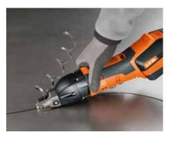
**Grinding without chips** Slitting shears are the right choice if swarf must be avoided when producing cut-offs and cut-outs. They cut a spiral chip from the sheet metal.
