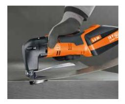
**Efficient and reliable** Sheet metal shears operate very efficiently and with no material loss at cutting speeds of up to 8 m/min.
