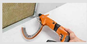
Produce screw fittings up to 6-times quicker thanks to magazine units
