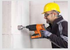
**Drilling** Produce 68 mm socket holes in masonry.
