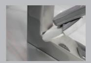
Fillet welds can be polished to a mirror finish with the felt disc and polishing pastes.
