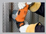
The large plunge depth and the rotating arm make it possible to access even hard-to-reach places.
