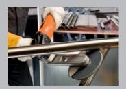
Heat discoloration can be quickly removed with the fine fleece disc without damage to adjacent components.
