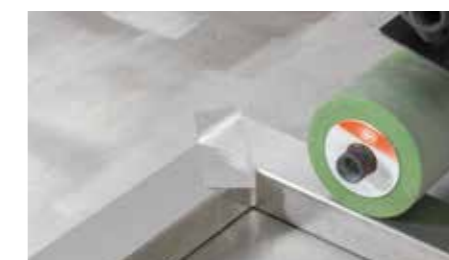
Cover and visually blend in the mitre joint when satin-finishing
