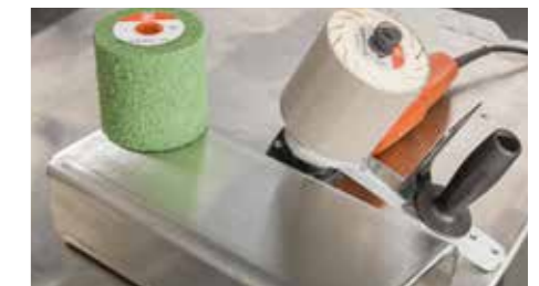
Further machining of the surface with K400, K800 and K1400, preparation for polishing
