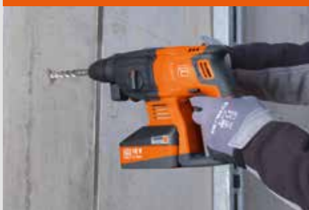
Hammer drill up to 20 mm in concrete.
