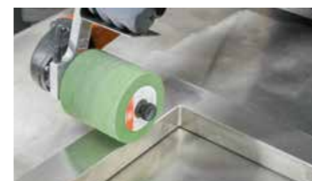
Satin finish without affecting the mitre joints
