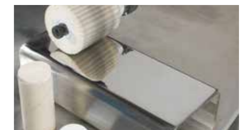
After processing with the colouring paste, optimum mirror polish on stainless steel surfaces
