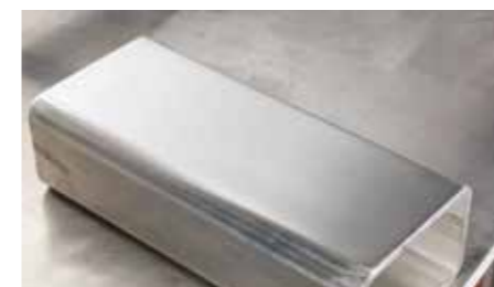
Surface pre-sanded to K1400, all scratches must be removed
