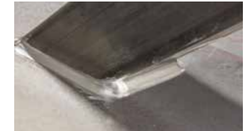
Even-looking surface and reliable removal of tarnishing on fillet welds
