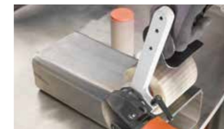
After applying the pre-polishing paste, produce mirror polish on the surface
