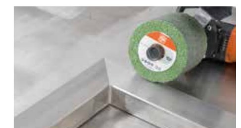
Clean grinding pattern in the mitre joint right up to the edge
