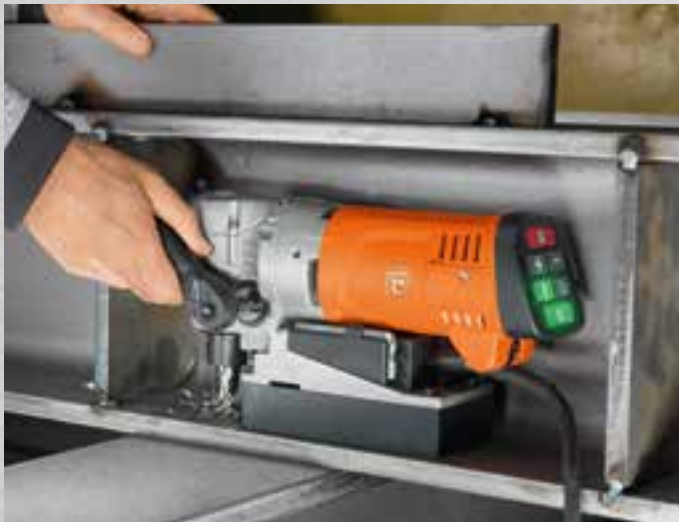
Working near edges and in tight spots
