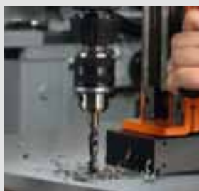
Twist drilling with drill chuck
