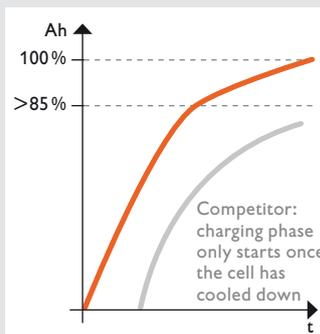
Shortened charge time: heat build-up is reduced thanks to high-quality battery cells with low internal resistance and the battery doesn't have to be cooled at outdoor temperatures of up to 45°C.
