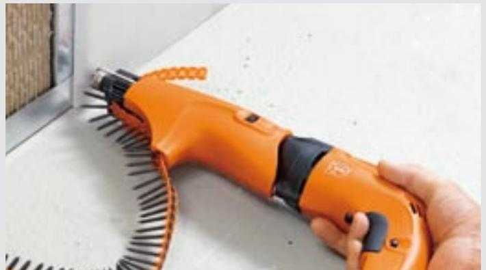
The FEIN magazine M55 with patented screw transport system delivers extremely reliable results – with all strips of screws from leading manufacturers. If required, it can be removed and cleaned tool-free. The screw length can be set to up to 55 mm and is suited to 1-layer to 3-layer sheeting.
