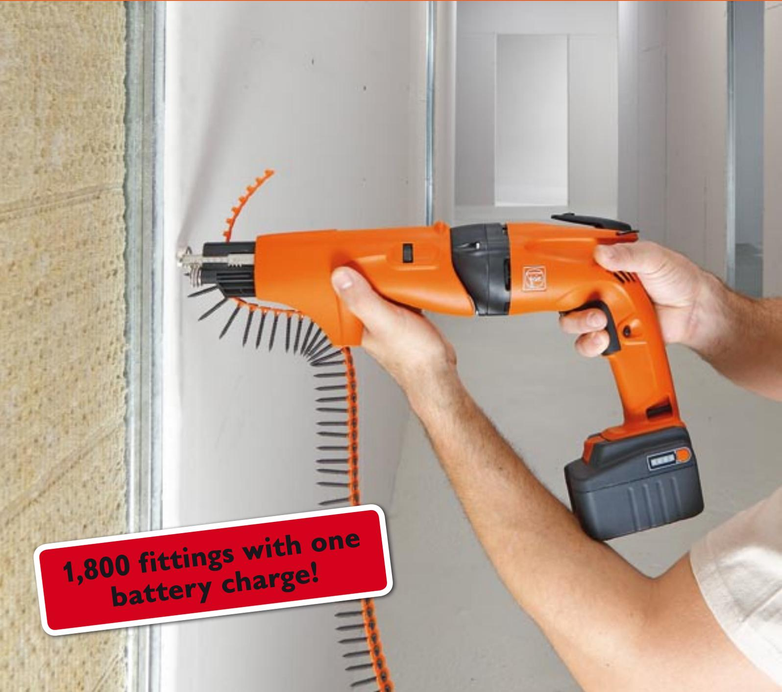
A person is using a bright orange FEIN dry wall screw gun on a wall. The gun is being held with both hands, and a long, flexible strip of orange and black screws is being fed into the front of the tool. The background shows a white wall and a window frame.
