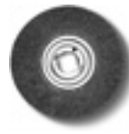
Steel wire brush Ø 250 mm x 60 mm, with very high wire drawing strength for highly efficient use, mounting hole Ø 51 mm. 0.2 mm thick wire for thin-walled pipes and profiles. 0.35 mm-thick wire for universal use. 0.5 mm thick wire for thick-walled pipes and profiles and great deburring results. Stainless steel version
