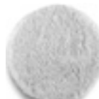
Bristle fleece Bristle fleece for cleaning or polishing boat hulls and decks, with a Ø of 195 mm for backing pads with a Ø of 170 mm, 6 38 06 187 01 0, M14 with hook and loop fastening system. For fibreglass anti-slip structures. Recommended working speed: approx. 500 rpm.
