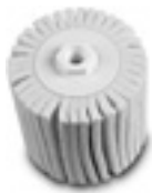
Felt lamella roller For polishing and pre-polishing stainless steel. Because of the lamella, the felt doesn't "burn" and polishing without streaks is possible. Only use with polishing paste (pre-polishing = pre-polishing paste, high-gloss polishing = colouring paste).
