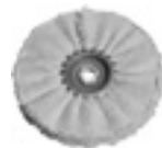
Felt lamella roller For polishing and pre-polishing stainless steel. Because of the lamella, the felt doesn't "burn" and polishing without streaks is possible. Only use with polishing paste (pre-polishing = pre-polishing paste, high-gloss polishing = colouring paste).
