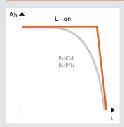
Effective from the first screw to the last: the new FEIN lithium-ion technology delivers constant power until the battery is completely flat.
