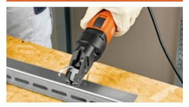
Cut varying thicknesses of profiles conveniently and safely – with FEIN nibblers and FEIN slitting shears.
