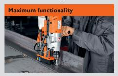
Core drill, twist drill, tap, countersink and ream - all with one tool. Maximum versatility in a wide range of applications.
