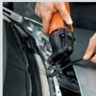
You can remove adhesive residue quickly, easily and effortlessly with the scraper blade. Recommended speed: setting 2–3.
