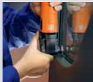
The curved type 072 cutter blade is ideally suited to cutting out side windows from the interior. Recommended speed: setting 3–4.
