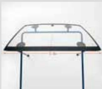
For the wire length, 5–6 times the overall width of the lower window edge is sufficient. A corresponding wire length of 2–2.5 times the interior width of the vehicle must be pulled into the interior using the awl.
