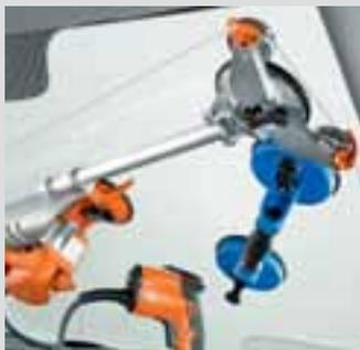
In rare cases the telescoping arm can slip on the window. This can be avoided with a normal suction lifting handle.
