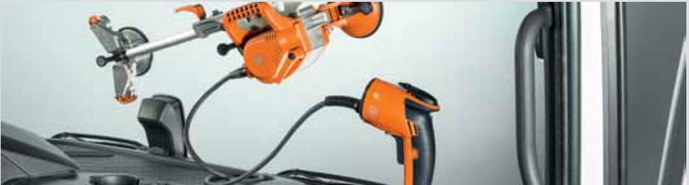
Truck windows can be safely removed with a single repositioning of the SUPERWIRE. The removal starts on the right side of the vehicle. This allows the window to be cut out to approximately the middle of the headliner. Then the SUPERWIRE must be moved to the left side.
