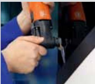
The type 081 and 216 straight blades remove cover strips neatly, safely, and quickly. In most cases, this allows the strips to be reused. Recommended speed: setting 3–5.
