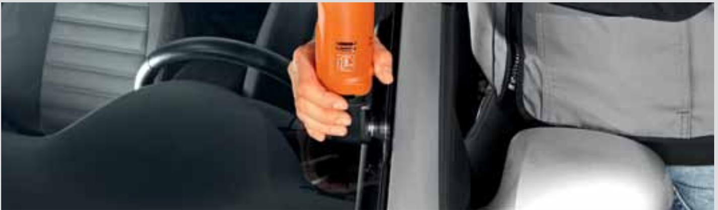
Extremely fast cutting: the type 207 L-shaped blade has an approximately 40% better cutting performance than a comparable U-shaped blade at the same speed setting. This is a great benefit when removing windshields from the outside. Recommended speed: setting 3–4.
