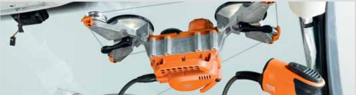
If the SUPERWIRE cannot be mounted with the telescoping arms, it must be repositioned once. After insertion of the wire, the SUPERWIRE is attached at the top right. The window is cut out as far as the upper edge and the SUPERWIRE is then moved to the left in order to cut out the remainder of the window.
