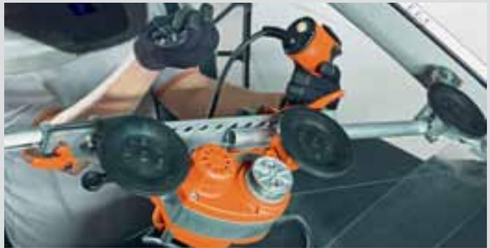
Thanks to motor power, the SUPERWIRE can be operated effortlessly by remote control from the interior or exterior.
