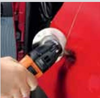
You can quickly cut normal auto body sheet metal up to 1/32" (1 mm) thickness as well as rigid plastic parts and GFRP with the HSS saw blades. The kerf is only 1/64" (0.5 mm) wide. Additional advantages: spark free cutting and customized plunge cut depths in the material.
