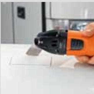
Cutouts in GRP and other resin-based materials can be precisely executed with the wide or narrow M-CUT HSS saw blades.
