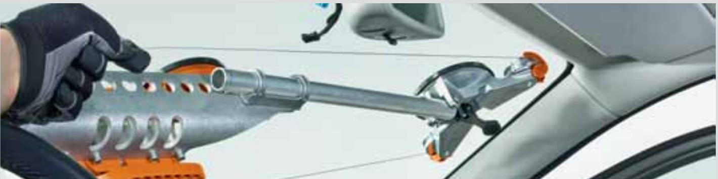
The telescoping arms are highly adjustable and therefore suitable for both side and rear windows as well as tightly curved windshields.
