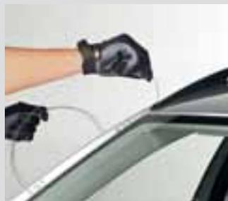
The wire is simply rolled under the molding. This way it is not damaged during removal and the window can be used again.
