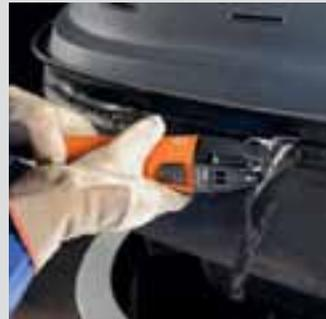
You can remove adhesive residue easily, neatly and quickly with the scraper blade – even in difficult-to-reach locations.
