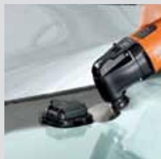
The new accessory range is also suitable for other tasks. For example, the light and windshield washer sensors frequently found in modern vehicles can easily be removed with the mushroom-shaped blade. Recommended speed: setting 2-3.
