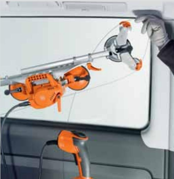
Easy removal of larger side windows without any repositioning. Always begin insertion of the wire at the top right.
