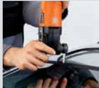
Encapsulated windshields and molded frames, including those with aluminum reinforcement, can be removed in one step using the L-shaped blade. Recommended speed: setting 3–4.
