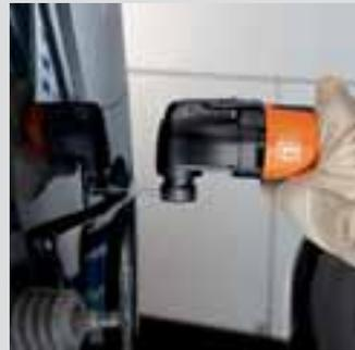
Type 207 and 209 L-shaped blades come into use on truck and bus windows with limited space between glass and frame. They will also cut through fixed strips easily and quickly. Recommended speed: setting 4–5.
