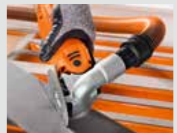
Perfect removal of dust with extraction device.
