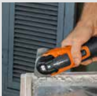
No risk of glass breakages thanks to oscillating motion.
