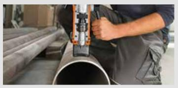
**Use with pipes** The magnetic contact faces have the shape of a prism. This ensures a secure hold, even when core drilling on pipes with a diameter of between 80 and 250 mm.
