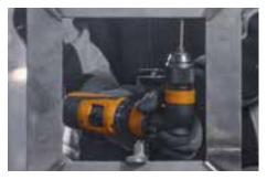
**Angled head** Metal angled head for drilling, tapping and screwdriving in confined spaces. All FEIN QuickIN accessories such as drill chucks, bit holders or socket adapters can be attached to the angled head.
