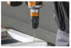
**SKE drill chuck** Drill chuck from Röhm with flat jaws and automatic re-tensioning. Prevents twist and tapping drills from slipping. Clamping width 1.5 to 13 mm. High concentricity of up to 0.35 mm for precise working.
