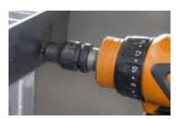
1/2 in socket adapter Socket adapter to hold sockets with 1/2" square holder.
