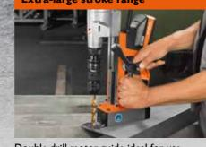
Double drill motor guide ideal for use with very large drilling tools. Continuously adjustable without the need for tools
